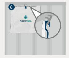
Hang the AbsorGel on the container lashing ring.
